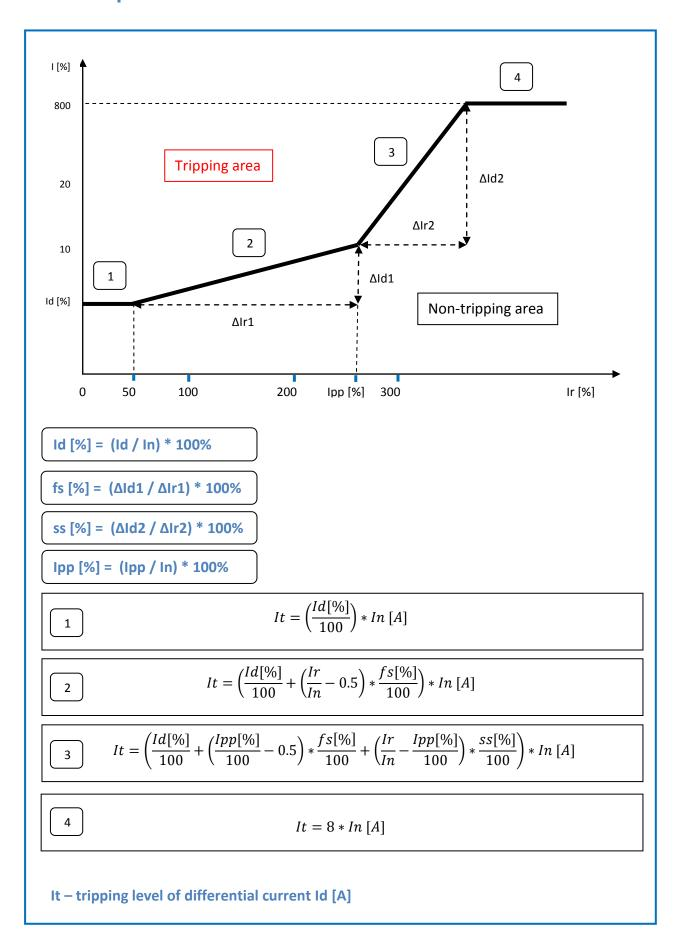
Current ratios must be set in accordance with ratios of the instrument transformers for each zone side.
